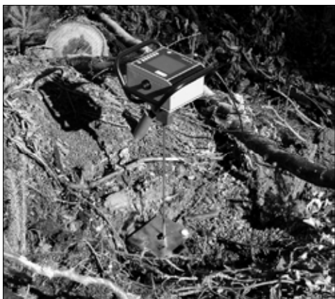
Obr. 2 Meranie zhutnenia v stope po podpere stroja Fig. 2 Measurement of soil compression
