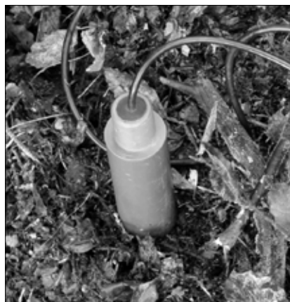
Obr. 3 Meranie vlhkosti vlhkomerom ThetaProbe Fig. 3 Measurement of humidity with ThetaProbe
